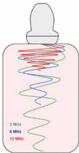
Figure 4: In the presence of higher frequency ultrasound waves and longer ultrasound path lengths, attenuation or energy loss is increased
